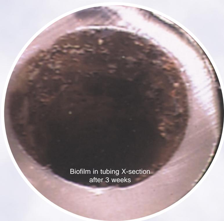
Biofilm in tubing X-section
